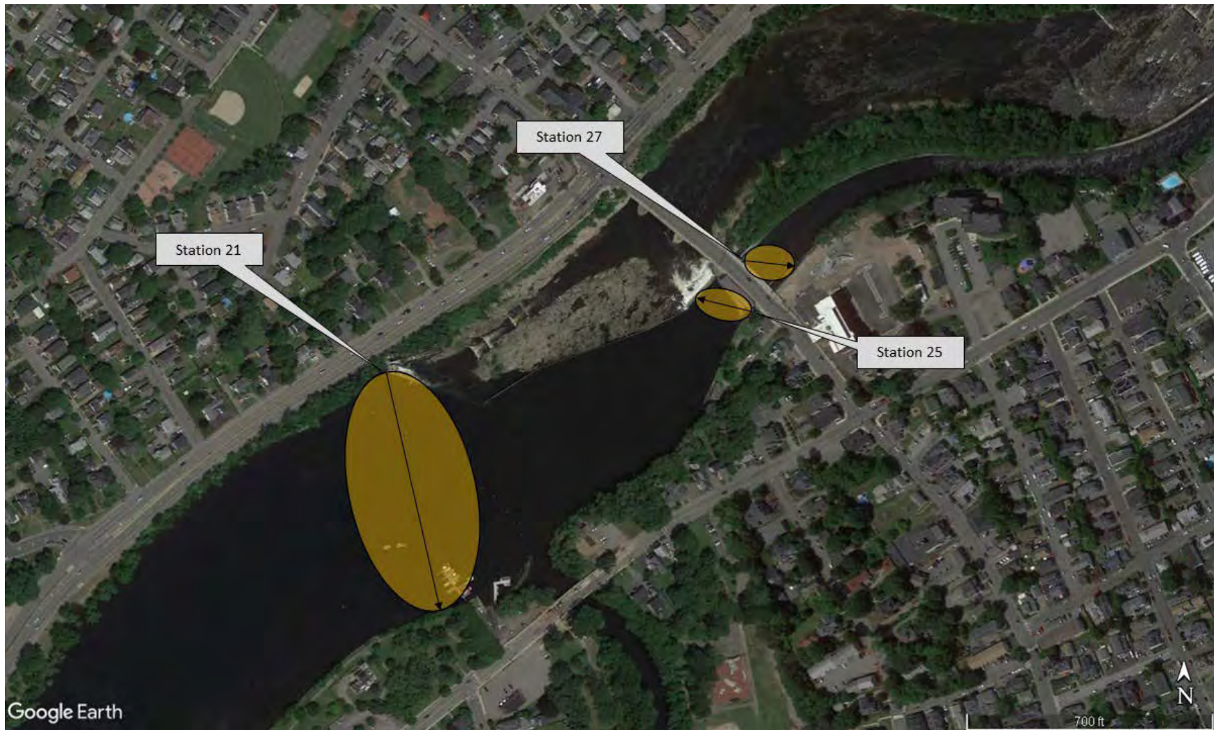
Figure 4–2. Locations and approximate detection areas for stationary radio-telemetry receivers installed upstream of Pawtucket Dam and at the Northern Gatehouse during the 2019 adult American eel downstream passage assessment at Lowell.
